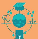
Circular process that delivers high food productivity in desert conditions. Water from fish ponds reused up to six times before discharge as nutrient-rich fertilizerirrigation water for vegetables, fruit tree and forage production. Producing yearly savings of 2,000 tons of fertilizers.
